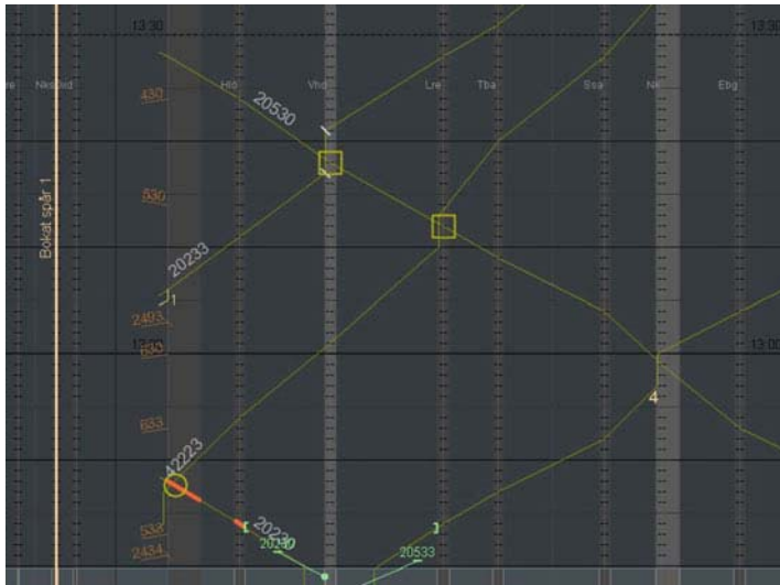
Fig. 5. Example of visualization of different types of conflicts. Conflicts are automatically detected and indicated. Yellow circles here mean a line conflict, e.g. two trains meet on a single track line. A yellow square means station track conflict, i.e. two trains are planned to use the same station track. During re-planning the removal or appearance of a conflict is visualized in real time (Color figure online).
